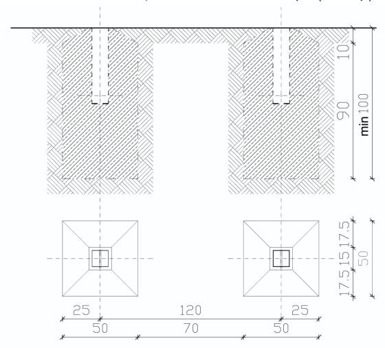
f) Slide the stand posts (1) into the concreted sleeves (6), tighten the M12x45 screws (8) into the locking mechanism and stabilise the stand posts in the sleeves
